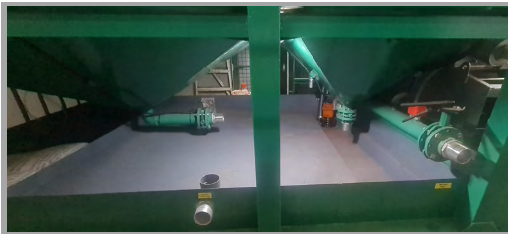
Liquid Sludge Collection Chamber with Auto Desludge Valves & Overflow
