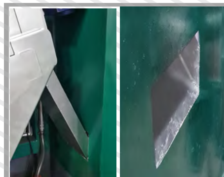
Sludge Cake Discharge Internal / External
